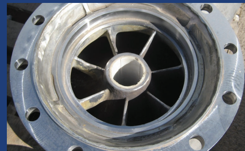
Water-lubricated Pump Bearing
