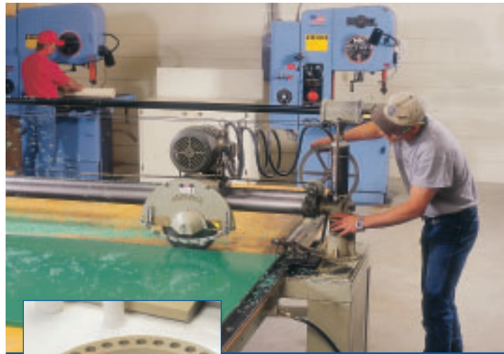
In-house skilled craftspeople create close tolerance cuts to within +/- .005, saving time and money.
